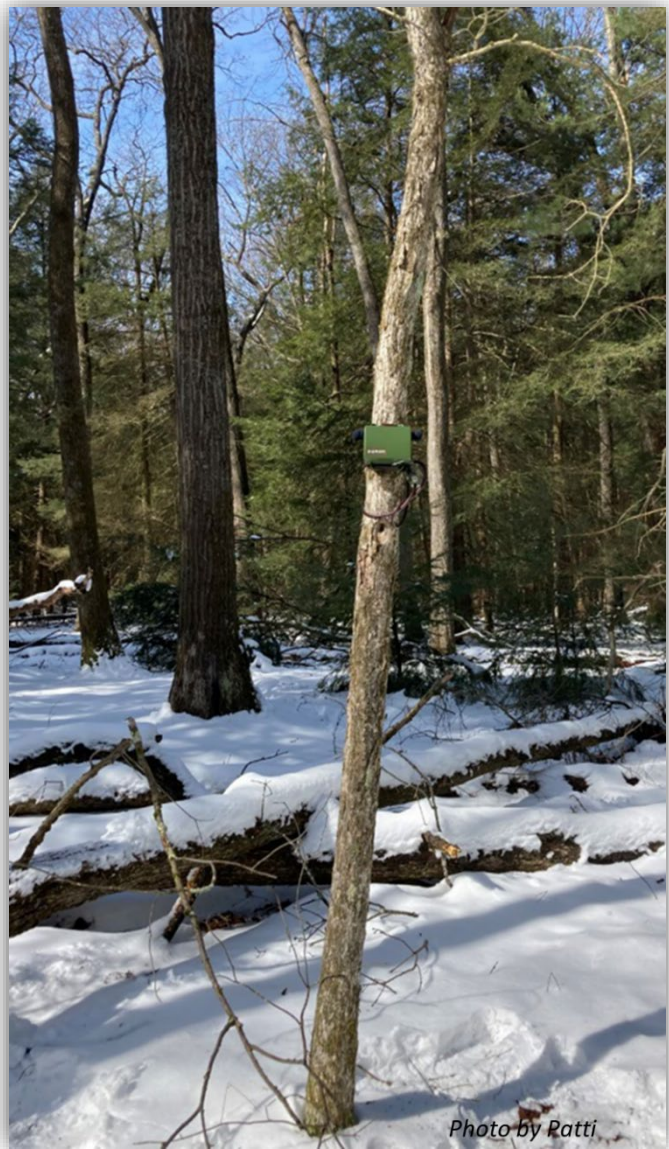
Figure 25. An autonomous recording unit (ARU) deployed in historic Northern Goshawk territory. Photo courtesy of the PA Game Commission
