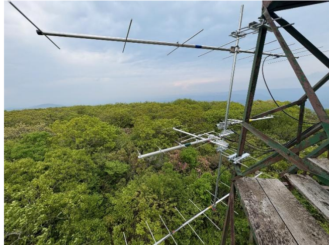
Motus antennas on a fire tower overlooking Warm Springs Mountain Preserve (TNC) in Bath County, VA.
